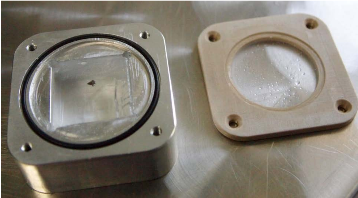
Sample cryo-holder with Vostok lake ice with inclusion
